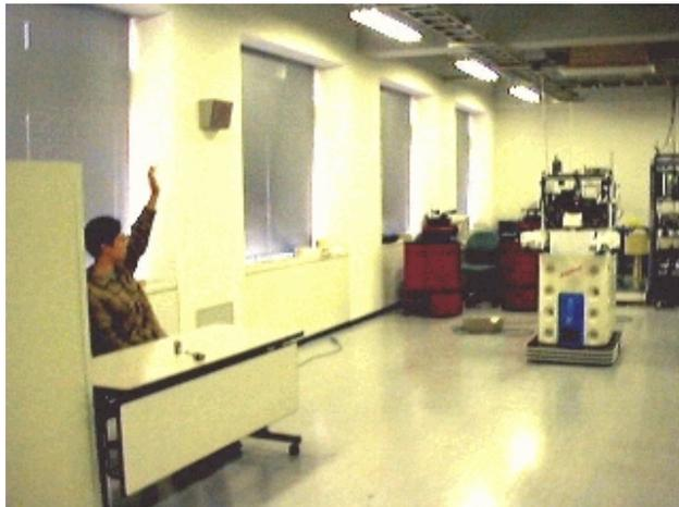
図 6: An example of loose interaction (a camera behind the robot detected human request and told the robot to go)
