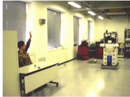
Fig. 10. An example of loose interaction (a camera behind the robot detected human request and told the robot to go)
